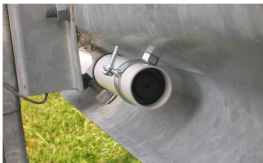
Figure 13. An INKE-1 mounted on W-shaped crash barrier in an interchange at fence end. The barrier also drives the sound well.
